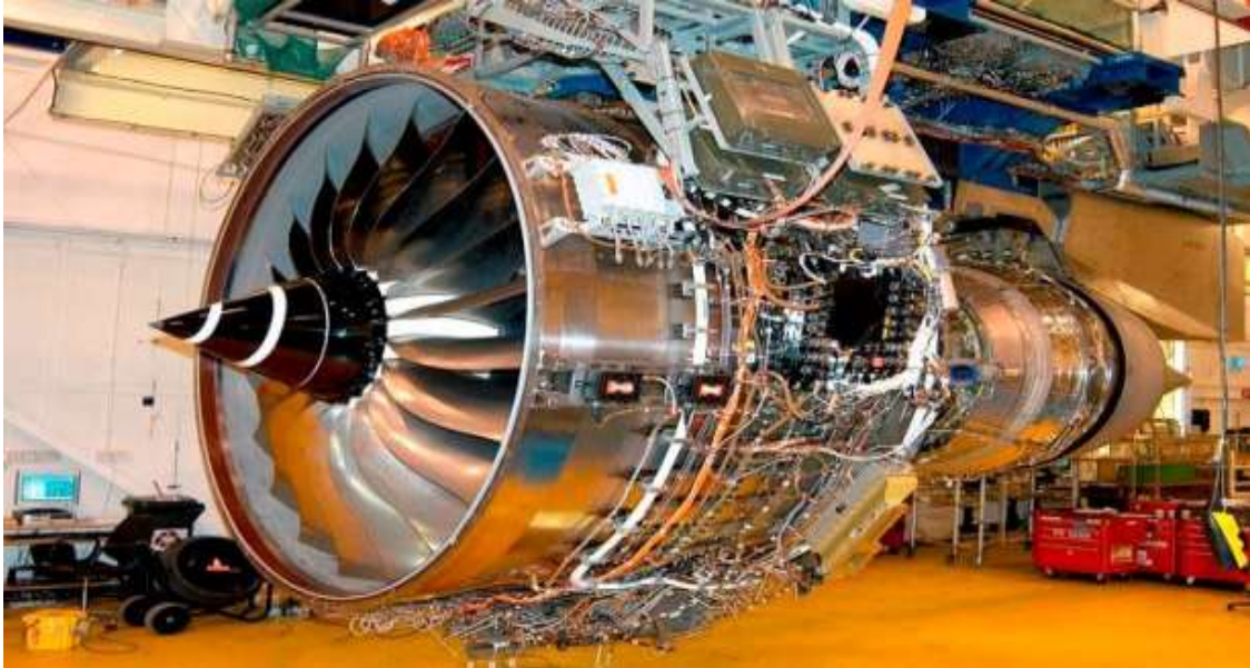
Figura 34: turbofan Rolls Royce Trent.
